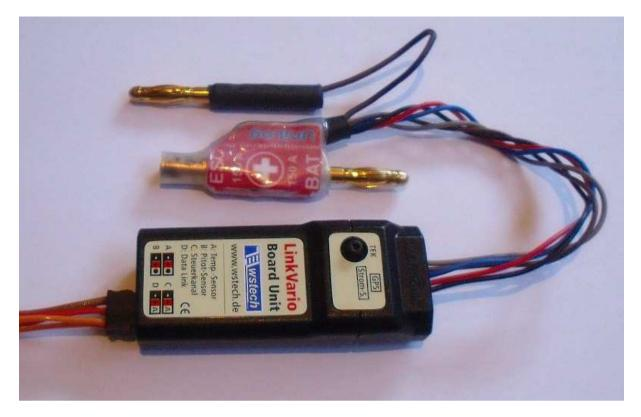
LinkVario with current sensor for monitoring of electric engines (voltage, current and capacity)
